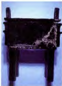
308: under ultra-violet radiation the false patina fluoresces
