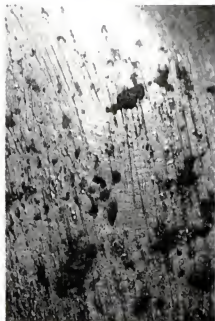
284: enlarged detail showing blisters characteristic of electroplating on poorly prepared surface
